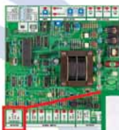
Receiver Connections on the Eagle Diamond Board
